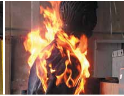
Non-FR 100% cotton after 480v disconnect arc flash.
